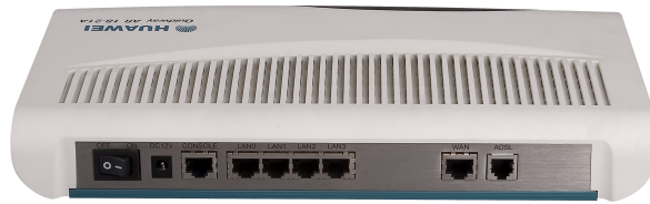
Figure 1-4 Quidway AR18-21B Rear View
