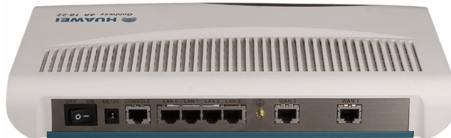
Figure 1-5 Quidway AR18-22 Rear View
